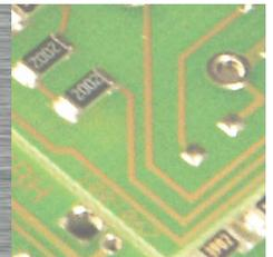
Input module for source or sink operation with 8 inputs, electrically isolated by optocoupler. Suitable for most electronic and electromechanical switching elements at 24 VDC.
