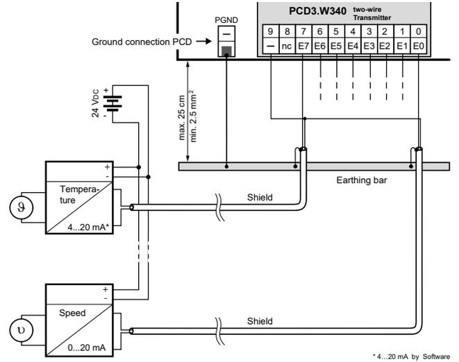
Two-wire transducers need a 24 VDC-supply in the measuring trunk.
