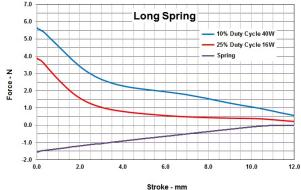
Typical Performance When Installed on Solenoid 195222-2XX
